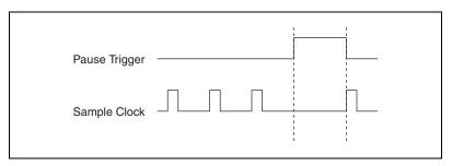
Figure 5-4. ao/PauseTrigger with the Onboard Clock Source
